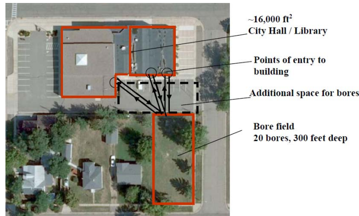
Figure 5. City Hall/Library Geothermal Bore Field Layout
